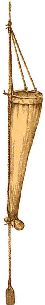
FIG. 14.—TOW-NET FIXED ON THE LINE ("Challenger").
