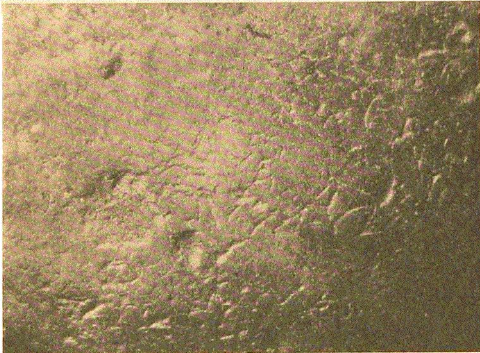
FIG. 147.—SURFACE OF SPECIMEN NO. 4 IN FIG. 146, ENLARGED TO SHOW "CHATTER-MARKS."
